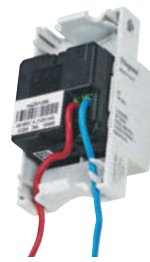
Wire up the power supply (screw terminals)
