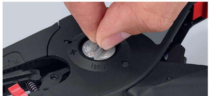
For special requirements, such as particularly hard or soft insulation materials, optimum fine adjustments can be made using the adjustment wheel with its tactile locking positions
