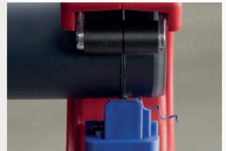
Segments as short as 10 mm can be cut. The spiral chip comes from chamfering.
