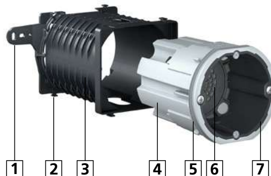
1 Fixing lug | 2 Snap-in connection for combinations | 3 Insulation thickness scale | 4 High-performance insulating components | 5 Sealing lips | 6 Moisture-controlling components | 7 Heat-conductive internal components
