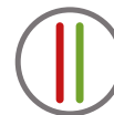
Longitudinal stripes of indelible color indicate the power of the protected cables
