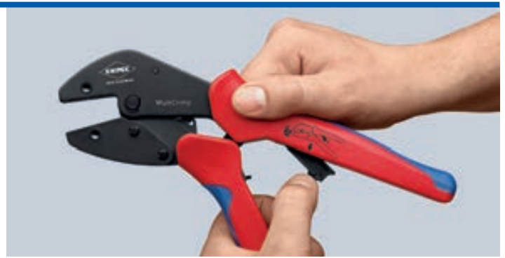
Changing position: service lever opens out for parallel jaw positioning
