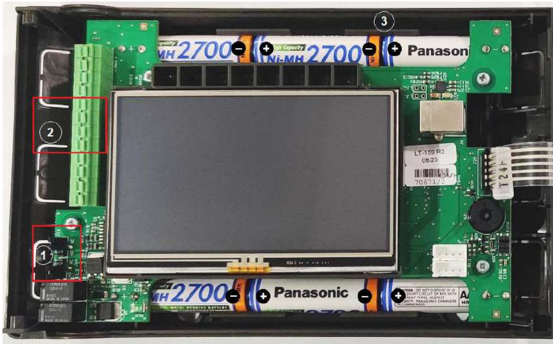
Fig. 17: LT-159 setup and connections overview
