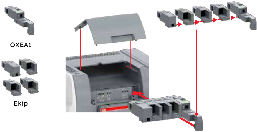
Fig. 9.6 Mounting of the auxiliary power supply module OXEA1 and Ekip –modules
