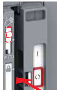
Fig. 8.11 Mounting the handle to the operating position; turn the slide switch to the Manual mode (Hand), lift the handle and place it to the operating position
