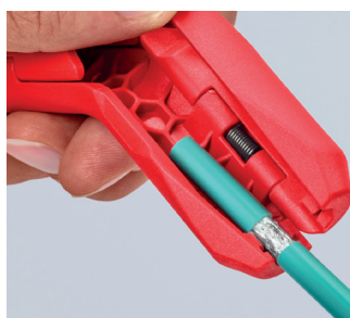
Stripping of a data cable
