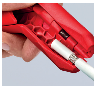
Stripping of a coax cable
