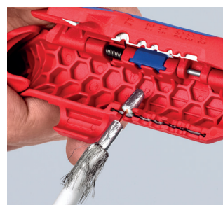
Stripping of a coax cable
