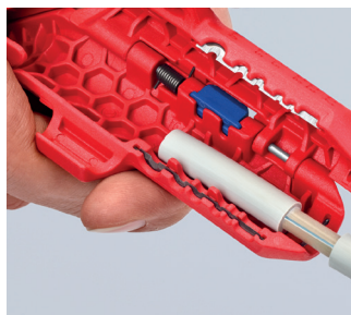
Stripping of a NYM cable
