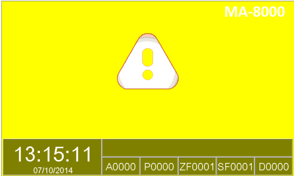
Fault display in stand-by condition
